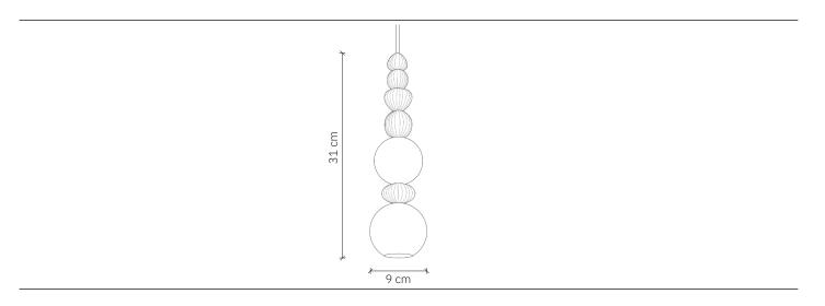
Model Bola Queen 2 Material Aluminium | Brass Finish Powder-coated aluminium Ø 9 cm, H: 31 cm **Dimensions** Power cord Fabric-coated black silicone - 120 cm Power supply 220-240V **Light Source** 6W LED (dimmable) Ceiling rose Hemisphere ceiling rose - powder-coated steel Weight 1,6 kg
