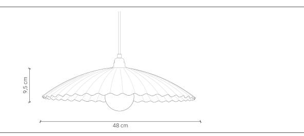
Model Fala Material Aluminium Finish Powder-coated aluminium Ø 48 cm, H: 9,5 cm **Dimensions** Power cord Fabric-coated black silicone - 120 cm Power supply 220-240V **Light Source** E27 max. 60W (not included) Ceiling rose Oval aluminium ceiling rose, powder-coated
