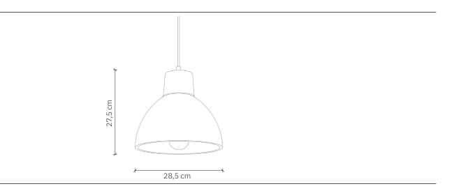
Model Korta 1 Concrete Material Hand-cast concrete Finish Coloured concrete **Dimensions** Ø 28,5 cm, H: 27,5 cm Power cord Customer's choice Power supply 220-240V **Light Source** E27 max. 40 W (bulb sold separately) Ceiling rose Flat concrete ceiling rose Ø 10 cm Weight
