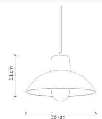
Model Korta 3 Concrete Material Hand-cast concrete Finish Coloured concrete Dimensions Ø 36 cm, H: 21 cm Power cord Customer's choice 220-240V Power supply **Light Source** E27 max. 40 W (bulb sold separately) **Ceiling rose** Flat concrete ceiling rose Ø 10 cm Weight
