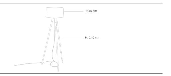
ModelMalta FloorMaterialConcrete | Alder wood | SteelFinishColoured concrete, raw alder wood, steel elementsDimensionsLampshade diameter: Ø 40 cm, H: 140 cmPower cordFabric-covered black silicone, 180 cm
