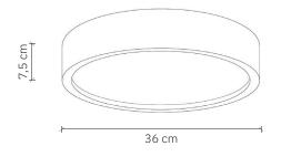
ModelPlan VelvetMaterialConcrete | GlassFinishColoured concrete, concrete covered with velvet structure, sandblasted glassDimensionsØ 36 cm, H: 7,5 cmPower supply220-240VLight Source18W LED, ~2700K (dimmable)Weight3,45 kg
