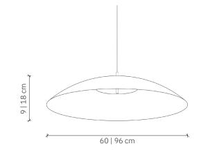
Model Telstar Velvet 60 | 96 Material Aluminium | Glass Finish Aluminium covered with velvet structure, sandblasted glass Ø 60 cm | Ø 96 cm, H: 9 cm | 18 cm Dimensions Power cord Fabric-coated black silicone, 120 cm Power supply 220-240V **Light Source** 24W LED, ~3000 K (dimmable) **Ceiling rose** Oval aluminium ceiling rose covered with velvet structure Weight 60: 2,5 kg; 96: 7 kg
