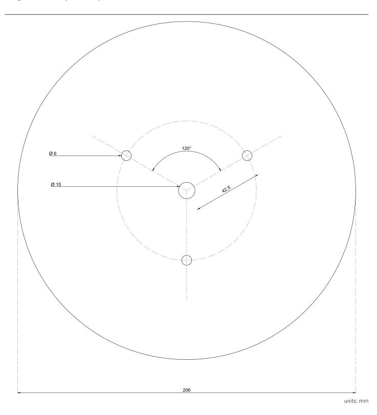
The drawing shows an aluminum plate with mounting holes, which should be attached to the wall using mounting dowels.
