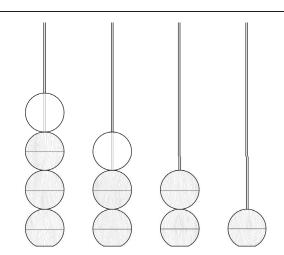
Model Woodoo Glass Material American walnut wood | Glass Finish Raw wood, sandblasted glass **Ball diameter** 9 cm Height Depends on number of spheres Black silikone 120 cm Power cord Power supply 220-240V **Light Source** LED 6W Ceiling rose Black steel hemisphere Weight
